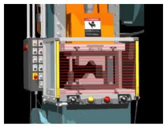
**Gates:** A gate locks in place in front of the point of operation of a press. Gates will not open until the machine has either completed its stroke (Class A Gates) or downstroke (Class B Gates).
