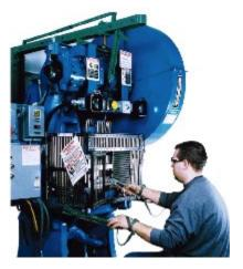
**Two-hand controls:** Two-hand controls require the operator to put constant and concurrent (both buttons pushed at the same time) pressure on controls in order to work a machine. If the operator removes their hands, the machine will stop before the operator can reach in. Two-hand controls must be tested frequently to ensure they are operating properly.
